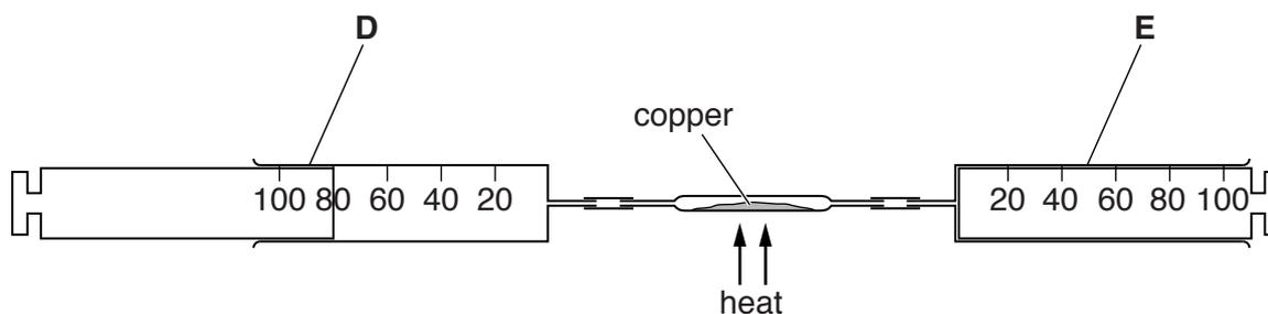
At the start of the experiment, **D** contains  $80\text{ cm}^3$  of air. The air is forced over heated copper into **E**. The air is then forced back into **D**. The process is repeated several times until the volume of gas forced back into **D** is constant. The gas is allowed to cool to room temperature before recording the final volume.
